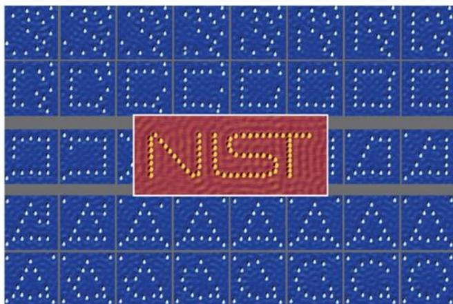
Automated assembly of individual cobalt atoms on an atomically flat copper surface into simple geometric shapes, a square, a triangle, and a circle. From left to right, each figure shows the configuration after each atom move. Image size 15 nm x 15 nm. Center: Perfect assembly of the NIST logo after four steps of automated assembly. Image size 40 nm x 17 nm. All images are shown in colored 3D top view with light shadowing with a height range of ~100 pm.
